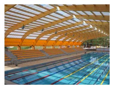
BDL<sup>®</sup> is a system of standing seam modular panels used to create vertical and sloped glazing. It is suited for a range of applications from curved skylights to interiors. Thanks to its wide variety of accessories, the system is complete, versatile, lightweight, and easy to install.
