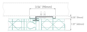
section panel / aluminum hook / panel joining
